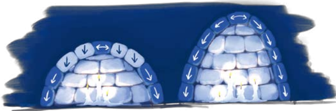
Figure 1. Force trend arrows showing the resultant force direction in a semi-circled shape with blocks of high tension and instability shown in white (left), and a parabolic arch shape (right) [5].
