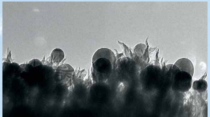
ORNL researchers developed a catalyst made of copper nanoparticles (seen as spheres) embedded in carbon nanospikes that can convert carbon dioxide into ethanol. (Photo credits: ORNL)
